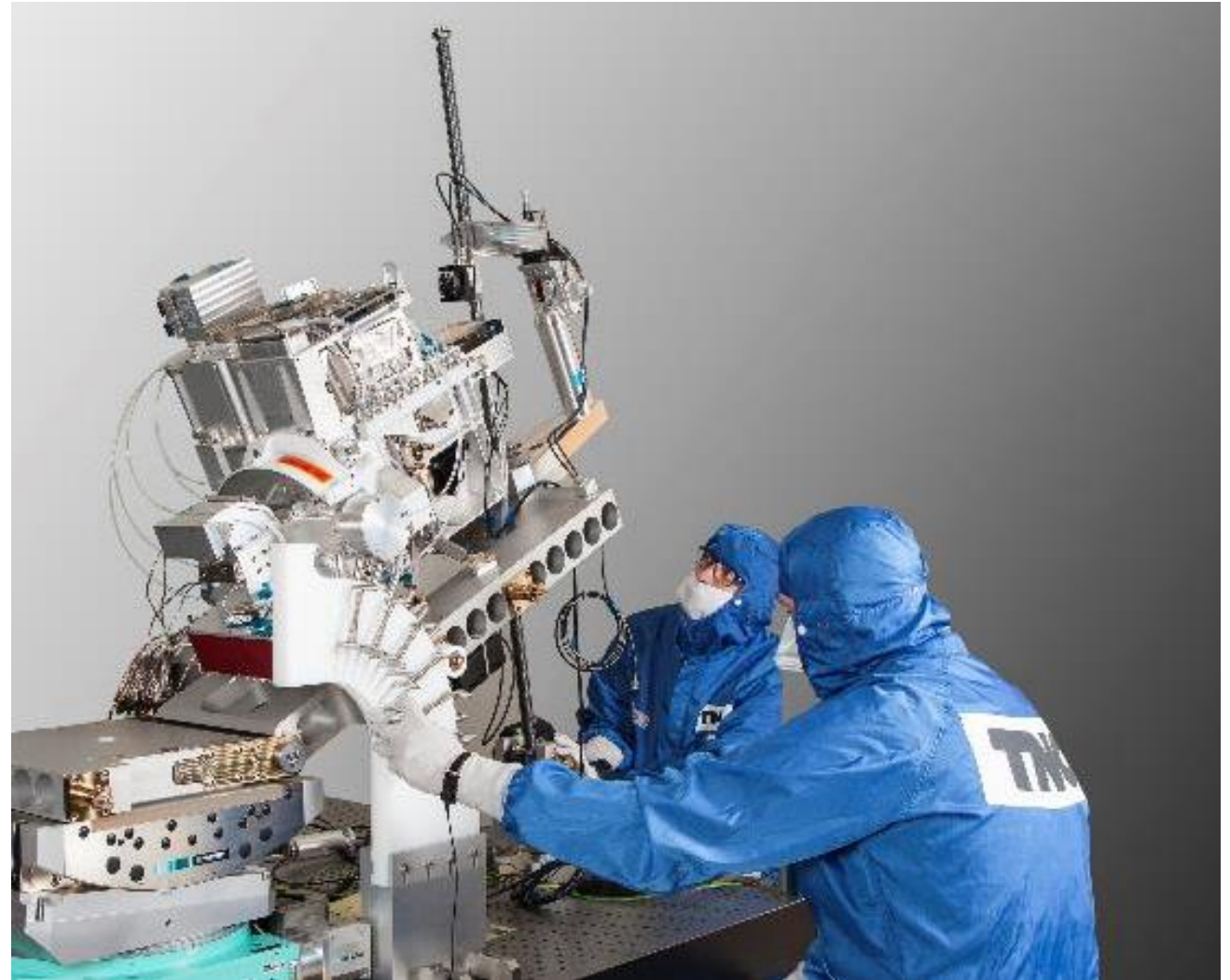
TROPOMI satellite instrument in TNO lab (TNO)
