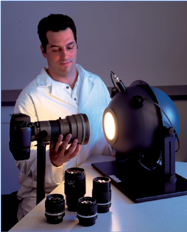
Figure 12: Integrating Sphere as a Source of Uniform Radiance Being Used for Correcting a Camera Image
